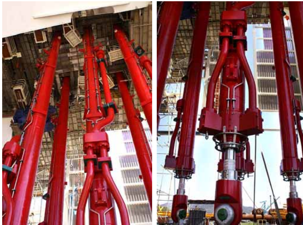
A core component of the riser tensioner system
