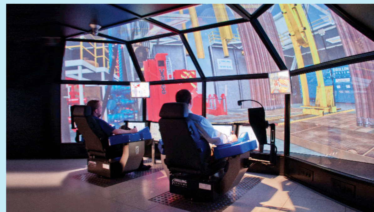
Drill crew being trained on a virtual reality drill simulator
